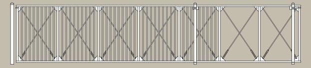
Secure-Trac® internal roller cantilever slide gates are produced using the highest quality materials and workmanship. The fully enclosed rollers eliminate safety issues commonly associated with external rollers and the gates are available to match each style of TangoRail® fence.
